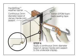
FIGURE 8 APPLY JOINT SEALANT
