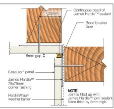
FIGURE 20C SEALANT FILL OPTION
