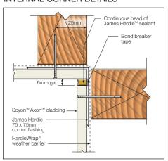
FIGURE 19 SEALANT FILL OPTION
