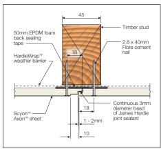
FIGURE 11 FIBRE CEMENT NAIL FIXING
