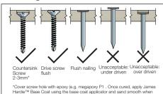
"Cover screw hole with epoxy (e.g. megapoxy P1. Once cured, apply James Hardie™ Base Coat using the base coat applicator and sand smooth when cured with 100-120 grit sand paper.
