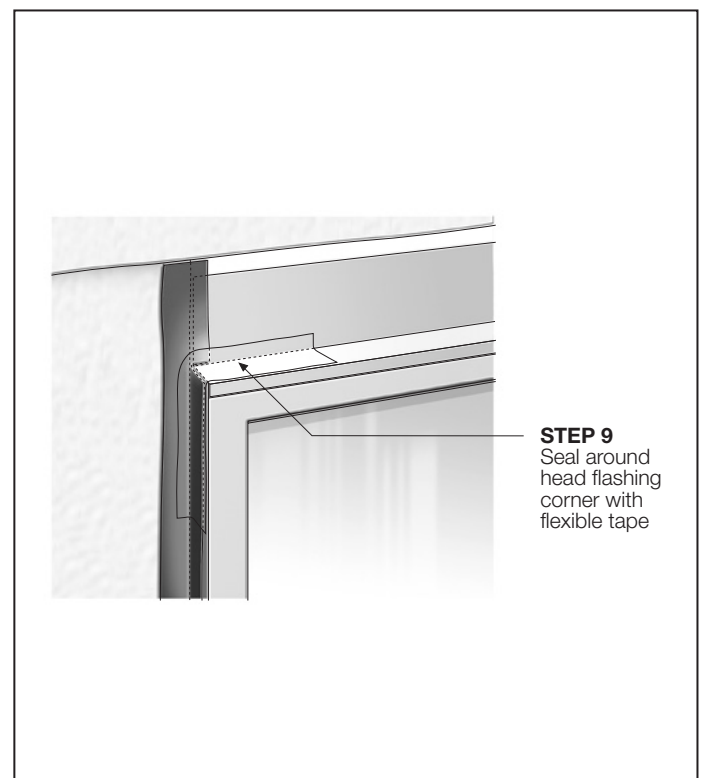
FIGURE 46 INSTALLATION OF WINDOW
