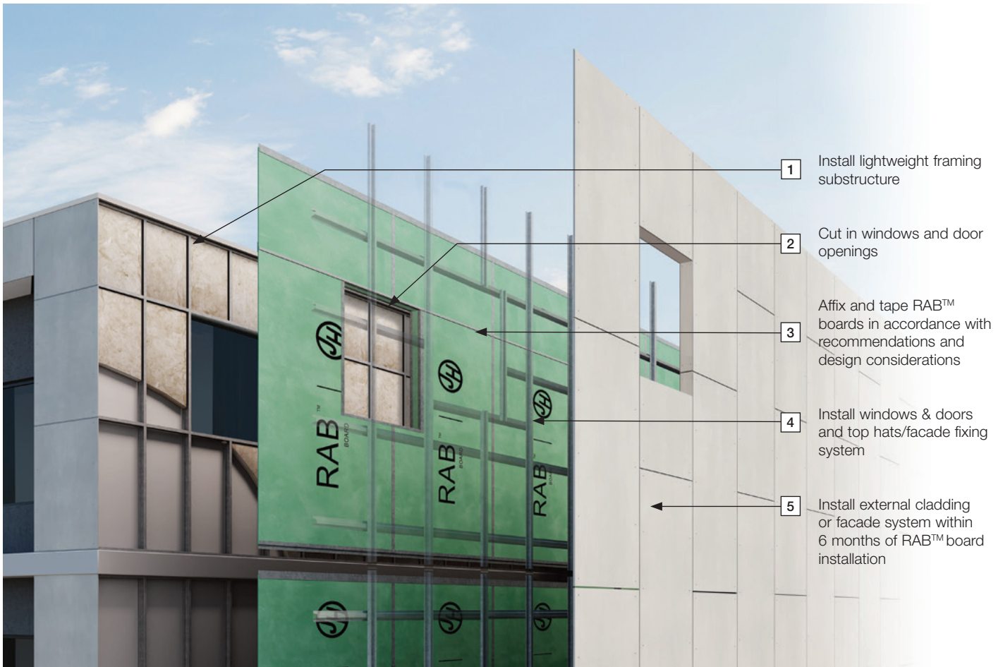
FIGURE 1 OVERVIEW OF THE WALL SYSTEM
