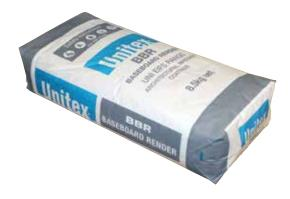
Unitex Uni-Dry Cote® BBR is a cement-based polymer modified, high performance, water resistant and adhesion promoting render system. This product is workable at thicknesses up to approximately 5-10 mm per pass.
