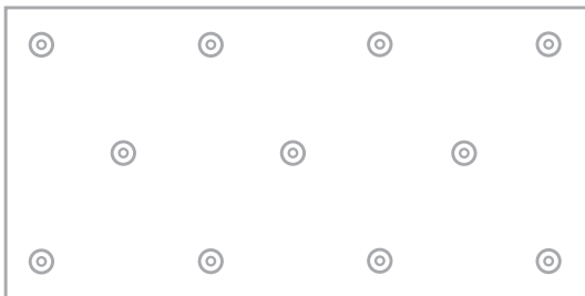
Figure 3 Fastener pattern (11 No. per board) Board size to 2400 mm x 1200 mm - 3.81 fixings / m 2
