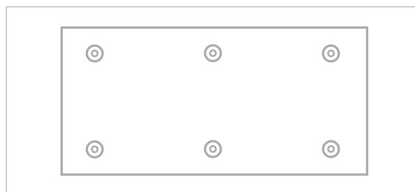
Figure 8. Fastener pattern (6 No. per board) 2270 x 1200 mm board - 2.2 fixings / m².
